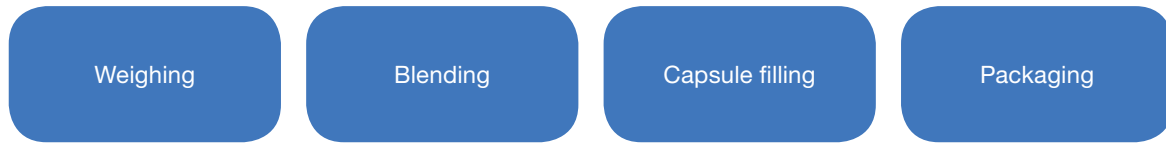
Fig. 5 Manufacturing steps for encapsulated products
