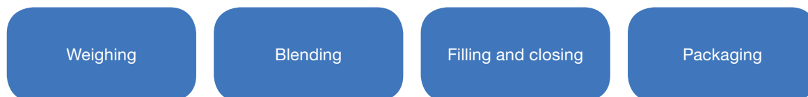
Fig. 4 Production steps for powders and powder blends
