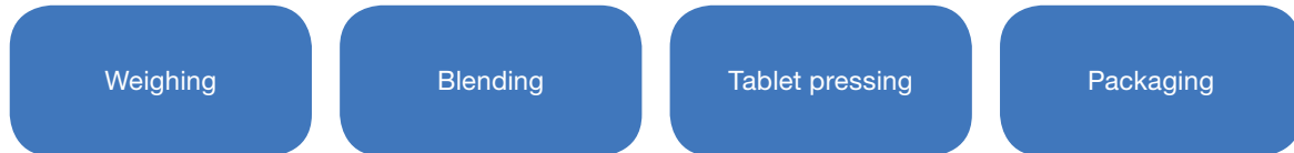
Fig. 6 Manufacturing steps for tableted products
